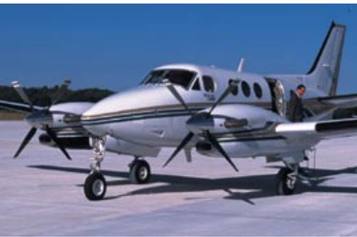
*This Raytheon Beechcraft King Air is a good example of a typical twin-engine turboprop used in on-demand air charter operations.*
